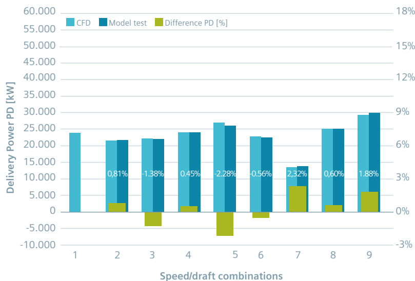
Comparison between the CFD analysis and model tests (image courtesy of DNV).
